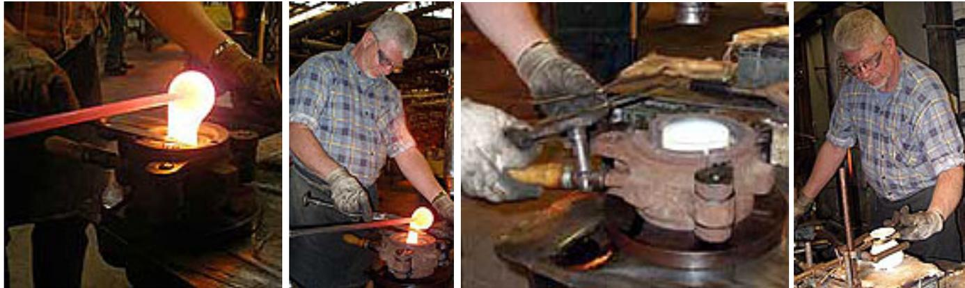
Using a punty, a gatherer brings molten glass and allows it to flow into a mould.
